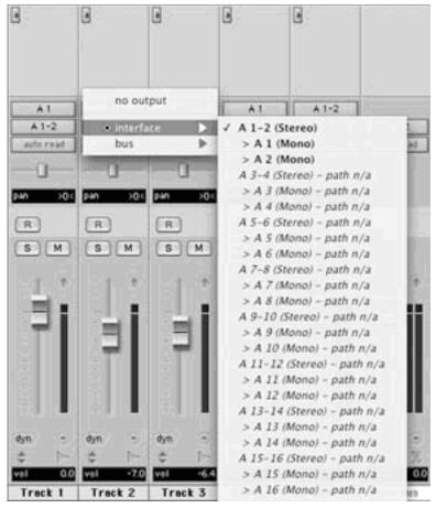
Figure 5. Pro Tools® track output selector, which routes signals to various processing buses and hardware outputs. © 2004 Avid Technology, Inc. All rights reserved.
